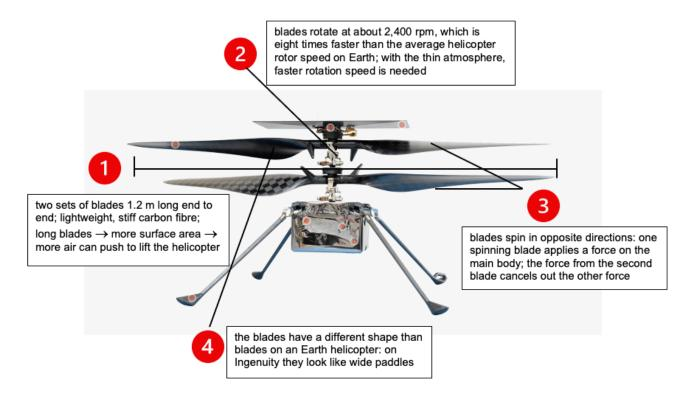
With such a thin atmosphere on Mars, the long, paddle-shaped blades and higher blade rotation speed are needed. Credit: image of Ingenuity: NASA/JPL-Caltech
